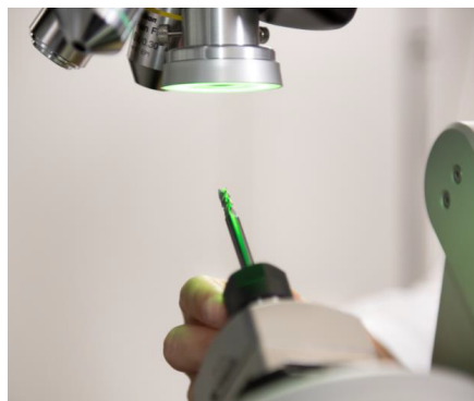
Motorized stage with 5-axis movement for automatic measure
