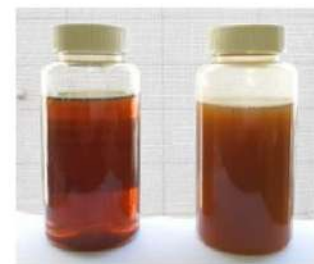
#5 Sample #3 Sample (32ppm) (1,528ppm) After 15 hours operation
